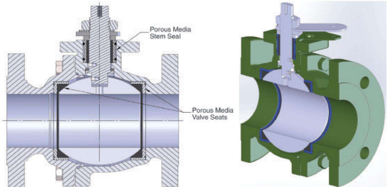
■ The New-Valve replaces traditional valve seats and stem seals with externally pressurized porous media and creates a seal of pressurized gas.
